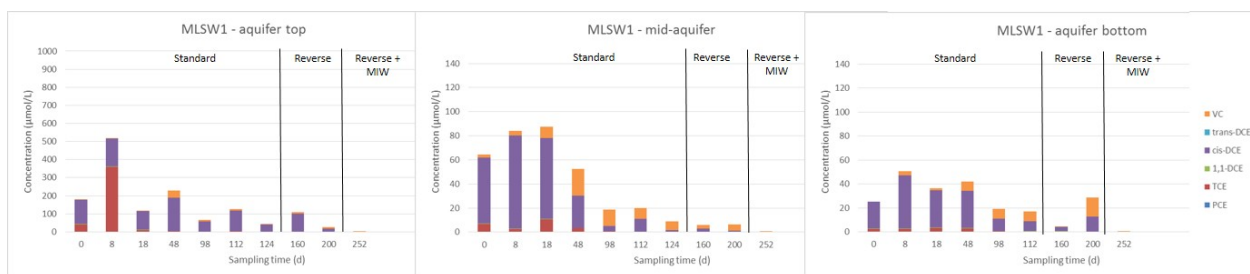
Fig 2: Molar CAHs concentration at different vertical sampling levels of MLSW1. Flow operation mode periods (standard, reverse) and C-MIX injection in the MIW is indicated in the graphs.
